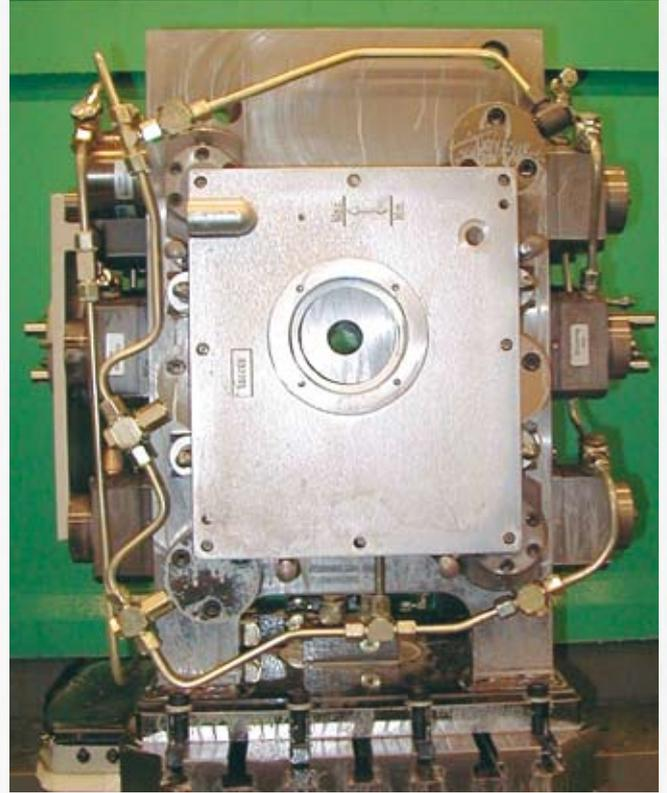
Gearbox clamping devices with and without workpiece, equipped with hydraulic pull-down clamps no. 6970 as clamping-element versions „centric“ and „eccentric“.
