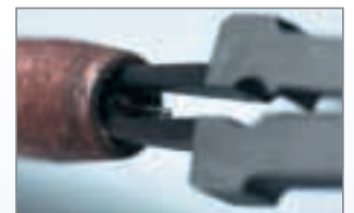
spatter removal from in and outside the nozzle
