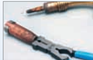
spatter removal from the nozzle end
