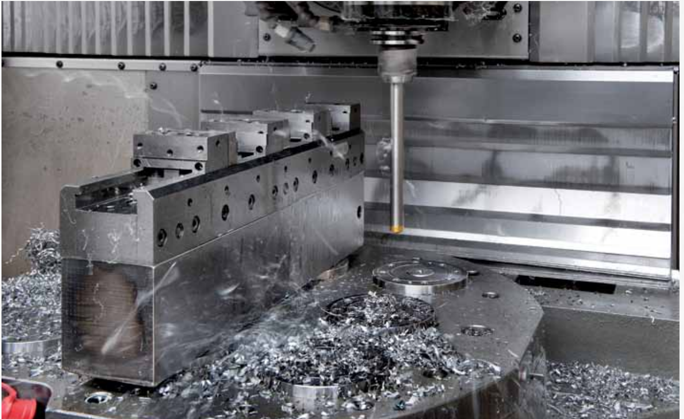
AMF-Clean-Stick in use: automated cleaning of clamping fixture and machine table
