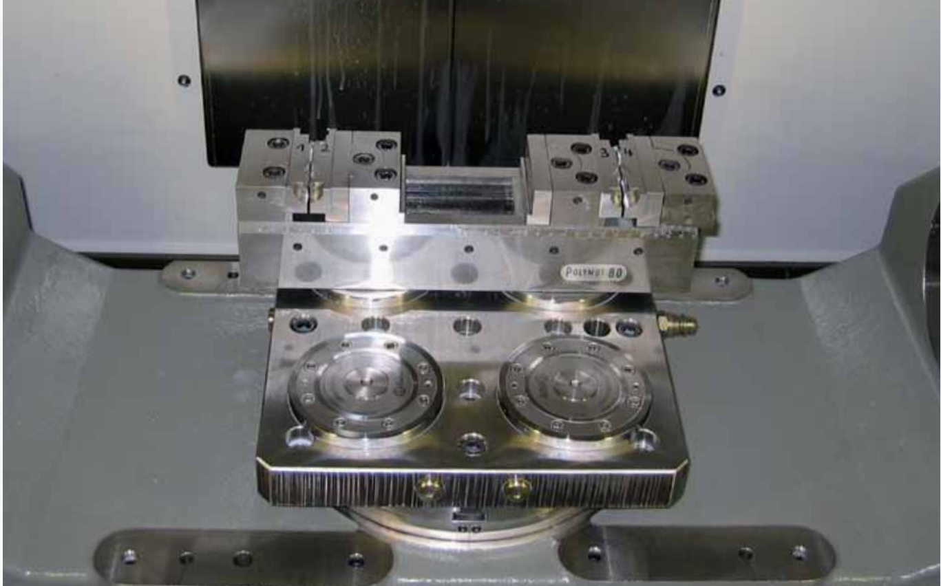
4-way clamping pallet mounted on round table for fast fixture changeover
