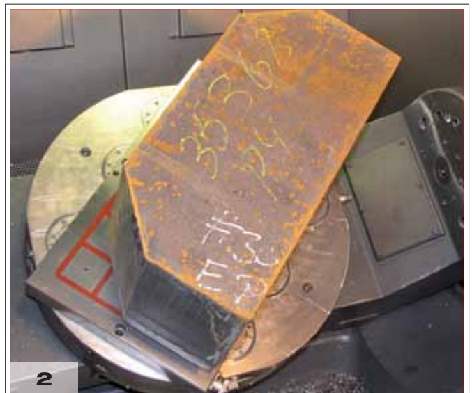
Flame-cut blank on the magnetic clamping plate, prepared for 5-side machining.
