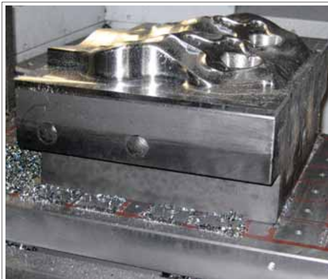
The mould part was directly clamped on the magnetic clamping plate and machined on all 5 sides with one clamping.
